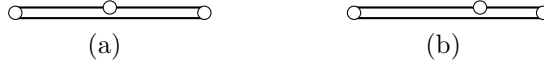
Figure 1: Collinear frameworks that are globally bearing rigid but not infinitesimally bearing rigid. Frameworks (a) and (b) are bearing equivalent and congruent and also globally bearing rigid. Observe, however, that the middle point can move along the line freely without changing any bearings, implying they are not infinitesimally bearing rigid.
